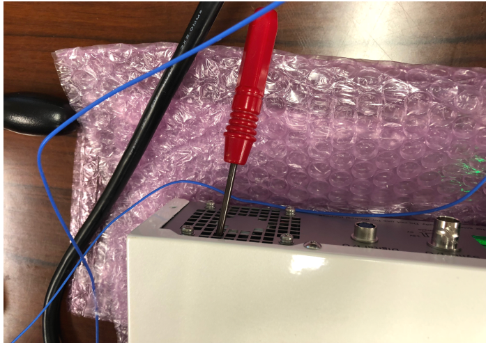
Picture2 Single Falure Condition (FAN Stopped by a stacking bar)
